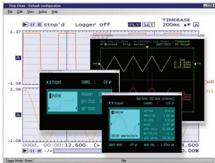
TracerDAQ provides four virtual instrument applications used to graphically display and store input data
