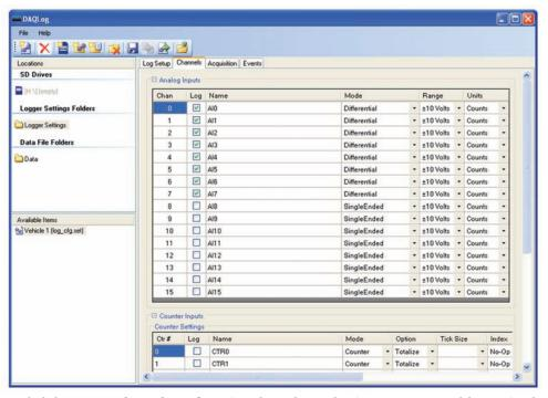
Included DAQLog software for configuration, channel setup, logging parameters, and data retrieval
