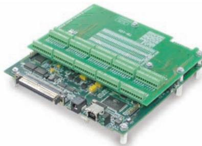
*USB-2527 with TB-101 screw-terminal board attached*
