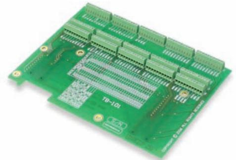
*TB-101, termination board with screw terminals, provides access to all USB-2500 Series I/O. The TB-101 mounts directly onto the board with included hardware.*
