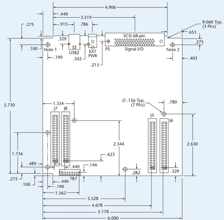
In general, all standoffs should be used to mount the board to a metal frame.
