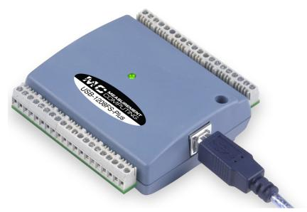
All devices in this series offer eight singled-ended or four differential analog inputs, two analog outputs, 16 digital I/O, and one counter input. Eight of the digital I/O on the USB-1208FS-Plus/1408FS-Plus can be used for high-current (24 mA) connections.
