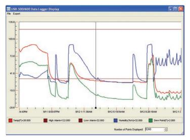
The included USB-500/600 Data Logger software displays recorded measurements in an easy-to-read chart. Movable markers isolate data values along with a time stamp. Temperature, humidity, dew point, voltage, or current measurements are displayed. In addition, high and low alarms are also shown.
