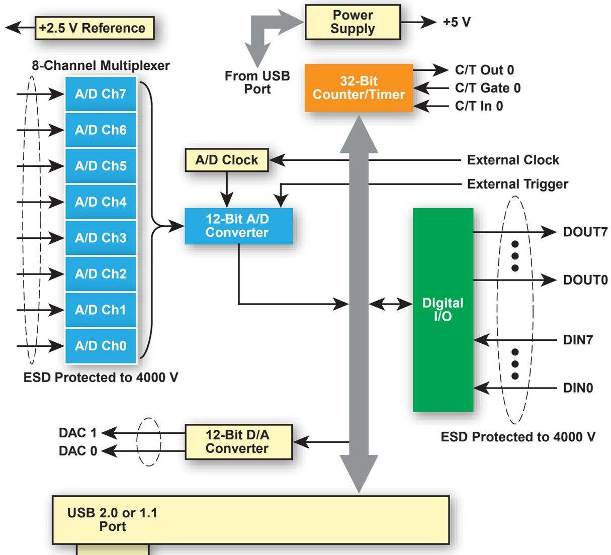
Figure 2. Block Diagram of the DT9812-10V, DT9812-10V-OEM, and DT9812A Modules.
