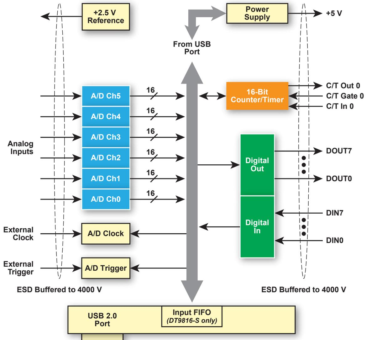
Figure 4. Block Diagram of the DT9816 Series Modules.
