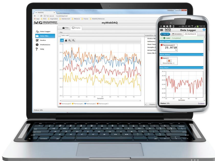
Device-independent operation lets you remotely monitor and control the WebDAQ 316 from any device with a web browser.
