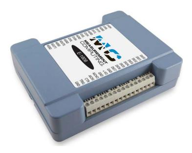
The E-1608 offers four differential or eight single-ended analog inputs, two analog outputs, eight digital I/O, and one event counter input.
