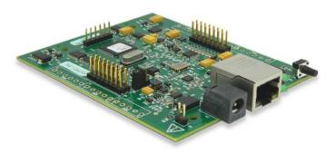
The E-1608-OEM has the same specifications as the standard device, but in a board-only form factor with header connectors instead of screw terminals.
