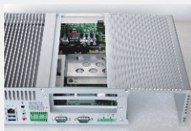
Fast disk and PCI / PCIe card installation, maintenance structure
