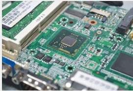
Onboard N2500 processor, power consumption 6.5W
