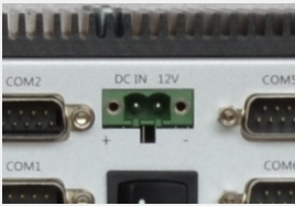
Phoenix terminal using fastening type power connector
