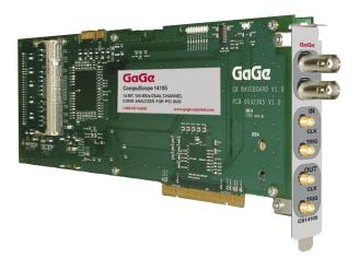
Digitizer module conceived and designed for critical communications and RF signal capture and analysis.
